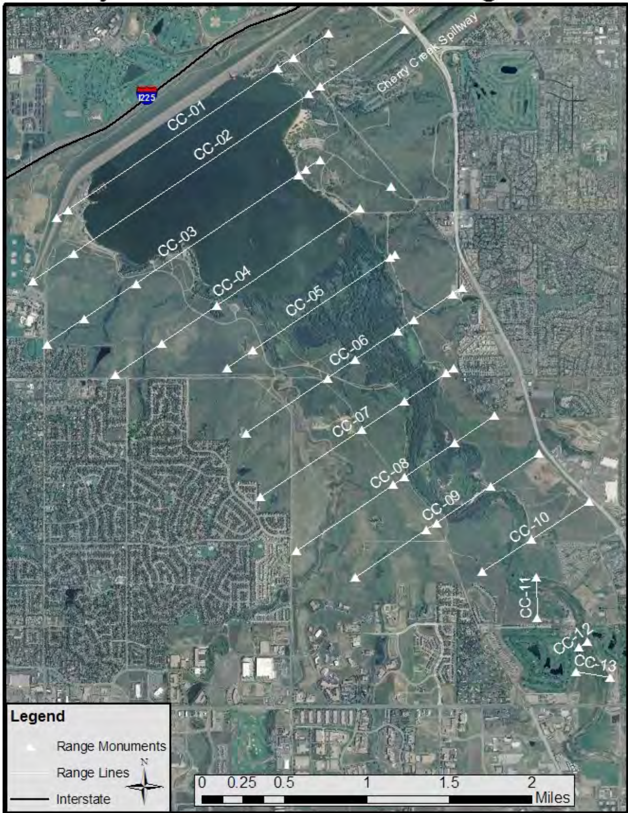
Figure 5-1. Cherry Creek Lake with Sediment Range Line Locations
