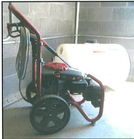
HIGH PRESSURE SPRAYER AND 30 GALLON WATER STORAGE TANK
