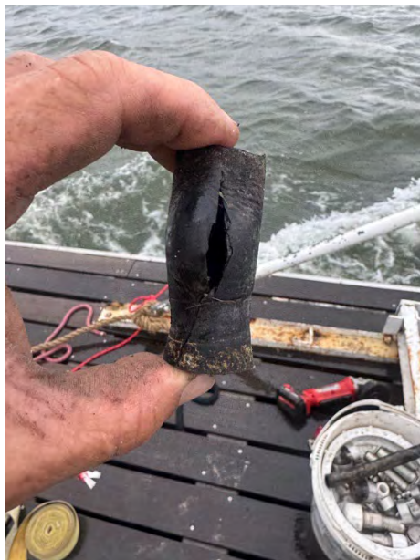
An example of a ruptured aerator hose
