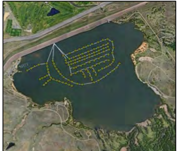
In-Reservoir Distribution System footprint – avoid boat anchors in this area.
