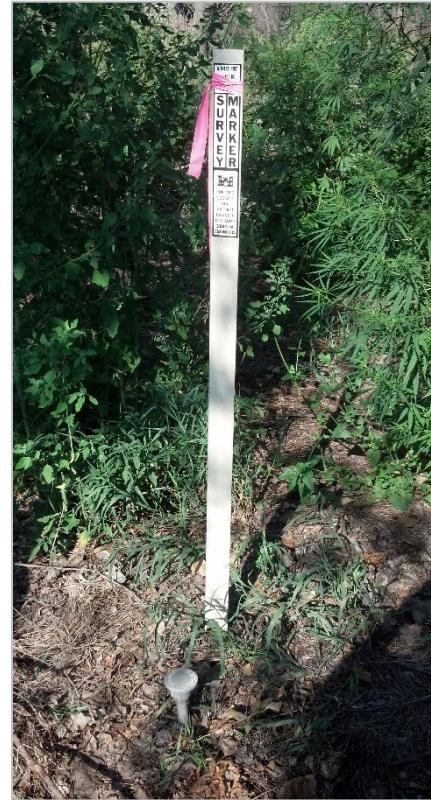
Figure 3-1. Example Survey Control Point and Witness Post
