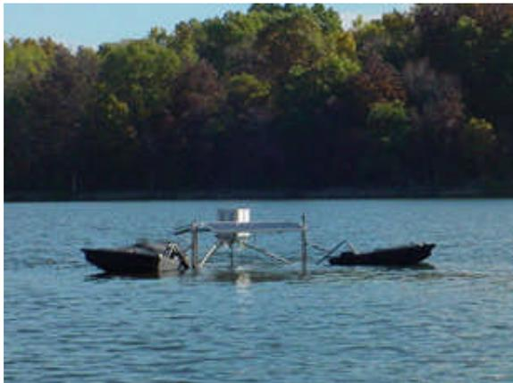
The SolarBee® is a solar powered circulator that floats on the surface and requires no external electrical power. The machine is 16-foot in diameter and can draw up to 10,000 gallons per minute from below and spread the flow across the top in near laminar conditions. Each machine can circulate flow up to 50-acres of surface area. Due to recent improvements in the motor, the system can operate 24-hours a day, although it is solar powered.
